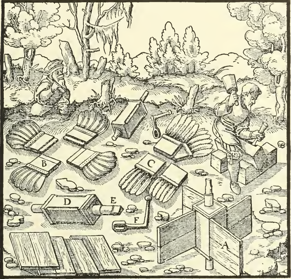
A—FIRST KIND OF FAN. B—SECOND KIND OF FAN. C—THIRD KIND OF FAN. D—QUADRANGULAR PART OF AXLE. E—ROUND PART OF SAME. F—CRANK.
